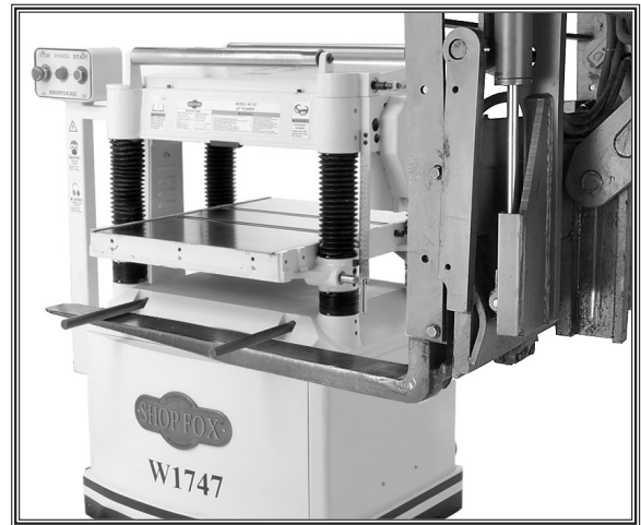
Figure 3. Example of planer being lifted using forklift.
